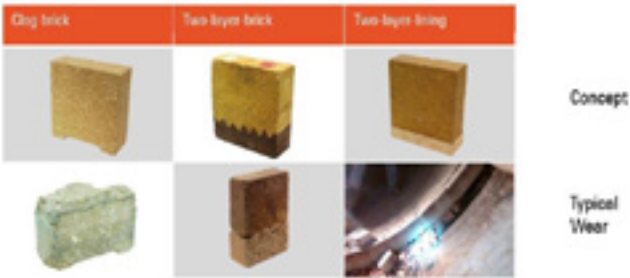
Fig. 3: Various concepts for thermal insulation of basic lined zones in rotary kilns
