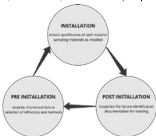
Fig. 1: Main steps for tracking the performance and quality of refractory linings in industrial applications.
