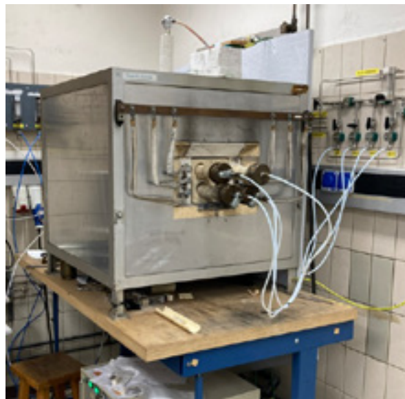
Fig. 3: horizontal tube furnace with gas mixing facilities
