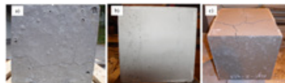
Fig. 6: Cubes (~75kgs, 300mm) after dry-out at 150°C for 12hrs: a) SF-6: 6% microsilica, b) SF-8: 8% microsilica, c) VF-6: 6% microsilica.
