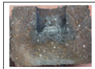
Fig. 10: Mg-Cr (20 % Cr_2O_3 ), slag is completely infiltrated
