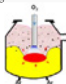
Fig. 1-1: Top Blowing Furnace Process (Conventional Furnace)
