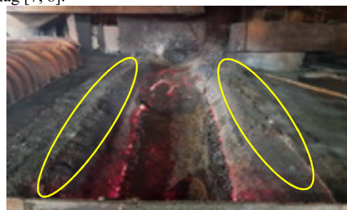
Fig. 1. Slag zone damage during main runner usage
