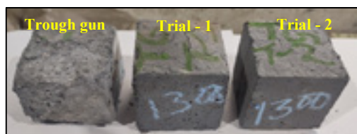
Fig.3: Samples appearance after blasting test at 1300°C
