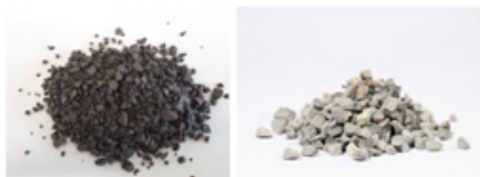
Fig. 3: Doloma grains from the new rotary kiln process [left] and the former shaft kiln process [right] showing darker colour due to higher iron oxide levels. Reprinted from [5] with permission.
