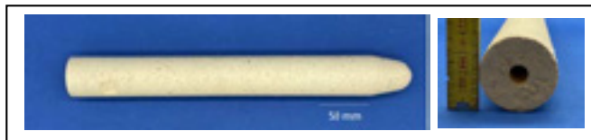
Fig. 6: Defect-free stopper rod prepared with coarse grained co-stabilized zirconia.
