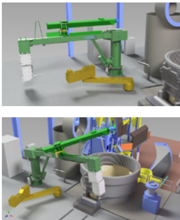
Fig. 8 a, b Gunning robot with laser scanner arm in parking, resp. scanning mode
