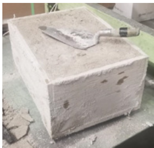
Fig. 1: Gunned sample formed inside shotbox
