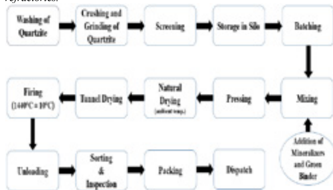
Fig. 3: Flow chart depicting the manufacturing process of silica refractories.
