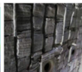
Fig.5: Interior refractory wall-temperature measurements (wall overheated and caused accelerated deterioration of fiber lining).
