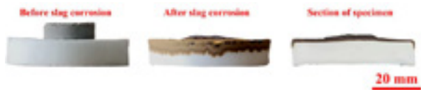
Fig. 7: Corroded CMA cylinder specimen
