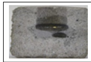
Fig. 12: Andalusite, DRI not, slag little infiltrated, microstructure on the right almost broken through
