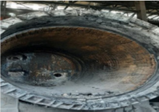
Fig. 7: Ladle condition during dismantling
