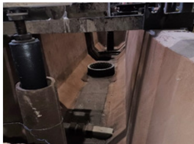
Fig. 7: Dry mix after baking thyssenkrupp Steel with the chimney technique
