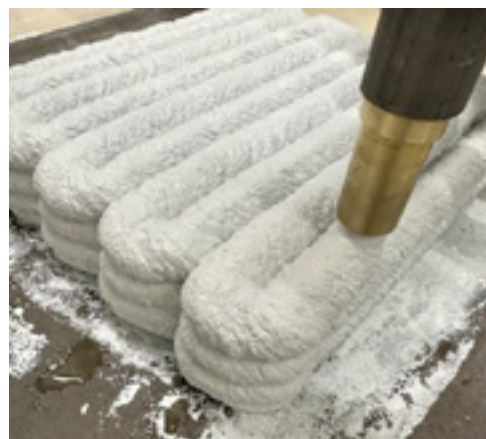
Fig. 3: Printing process of a cuboid with a dimension of 350 mm x 290 mm by layer-on-layer construction (10 layers in x-, y-axis and 5 layers in z-axis) with the large-scale printer after the scheme shown in Fig. 2. \text{Li}_2\text{CO}_3 was used as setting accelerator and directly added after nozzle exit.
