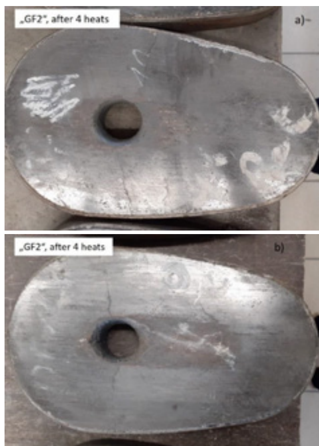
Fig. 8, a)+b): appearance of quality "GF2" after 4 heats
