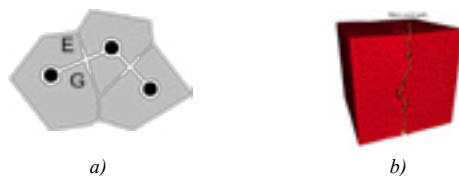
Fig. 4: Description of a) Lattice spring model b) Surface crack with polyhedral element [7]
