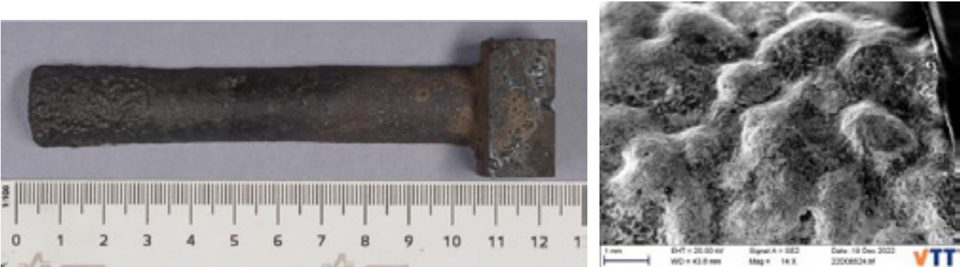
Fig. 3: Refractory finger after testing in slag contact and SEM image of the surface with slag reactions.
