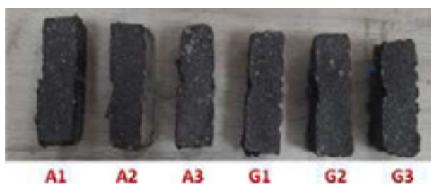
Fig. 5: Photographs of the corroded samples after performing a slag corrosion test in the induction furnace.
