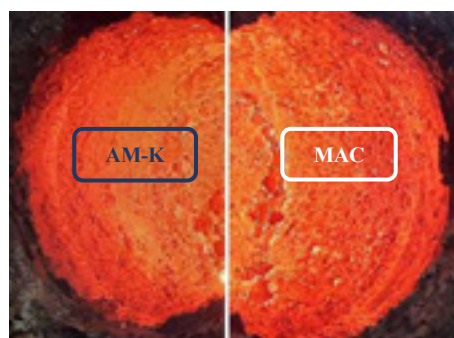
Fig. 6: Ladle barrel after 180 heats, with a better coating and insulation protection for the AM-K lining with the zero carbon technology concept.
