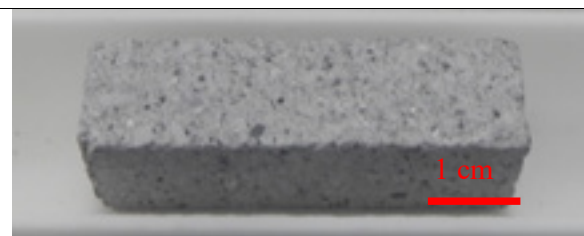
Sample of chamotte fireclay brick after test (100% CO)
