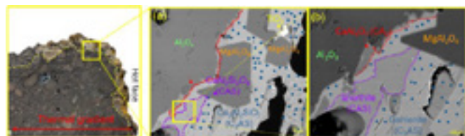
Fig. 2: SEM-BSE mode images of hot face of sample A-2, low magnification (a) and high magnification (b).
