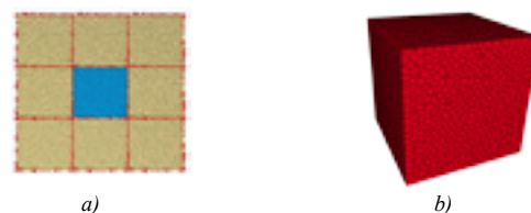
Fig. 7: Boundary condition a) Free boundary [8] b) Periodic boundary [1]
