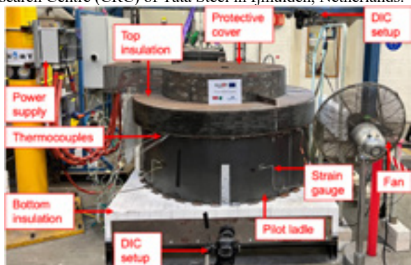
Fig. 3: Experimental setup of the pilot ladle.
