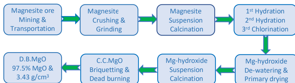
Fig. 1: Flow chart of magnesia purification and densification
