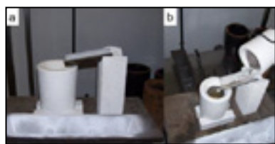
Fig. 1: Setup of the casting test before (a) and during casting (b) of molten aluminium.
