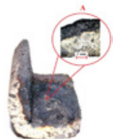
Fig. 2: Treated refractory pad modelling converter lining (30x30x30 mm), A – depth of slag penetration into the refractory.
