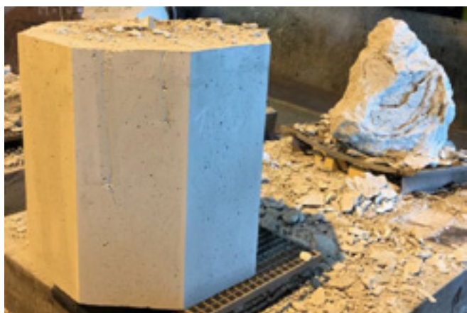
Fig. 7: Result of a large-scale fast heating test with different pre-shaped castable to 800 °C. Increasing steam pressure led to a total collapse of the sample on the right side.
