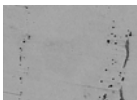
Fig. 5: Banded distribution of typical inclusions in original steel samples
