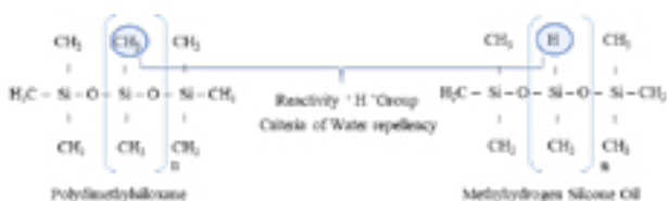
Fig. 2: Chemical Structure of the Silicone oil
