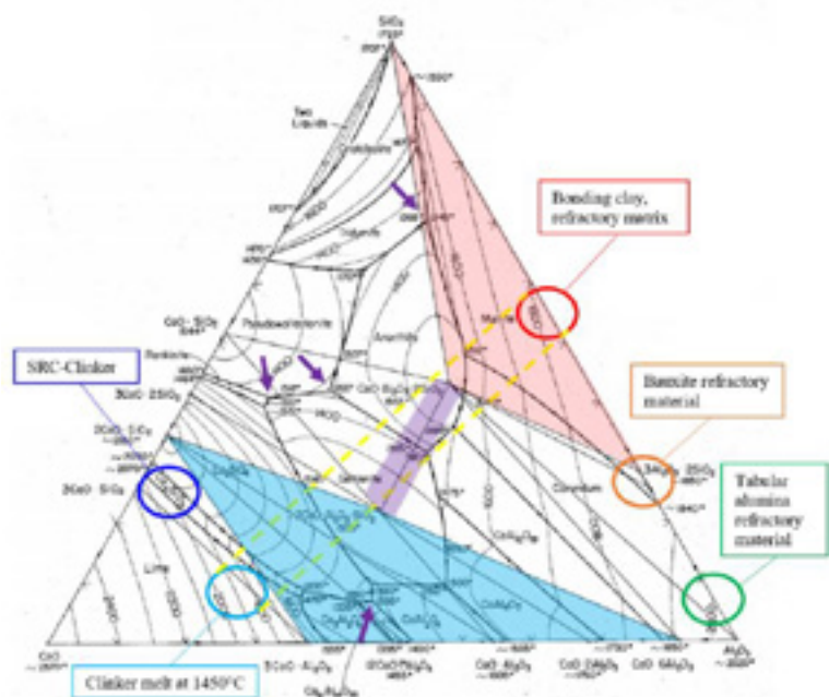
fig. 13: Ternary system \text{CaO-Al}_2\text{O}_3\text{-SiO}_2 [2] with plotted composition of the used materials and a typical clinker melt composition at 1450 °C [3] (circles). First reactions were assumed and observed between the refractory matrix (red circle) and CaO coming from the eutectic clinker melt, which is formed in every clinker [3] (light blue circle). Considering a diffusion of \text{Ca}^{2+} , all compositions between the tie lines (yellow dashed) of both materials exist at the same time. These coexistent compositions in the reaction zone plot in the systems belite-calcium aluminates-gehlenite (blue area), gehlenite-anorthite (purple area) and anorthite-mullite-cristobalite/glass (red area). Relevant eutectics of the locally formed composition are in the range of 1270 - 1350 °C (purple arrows).
