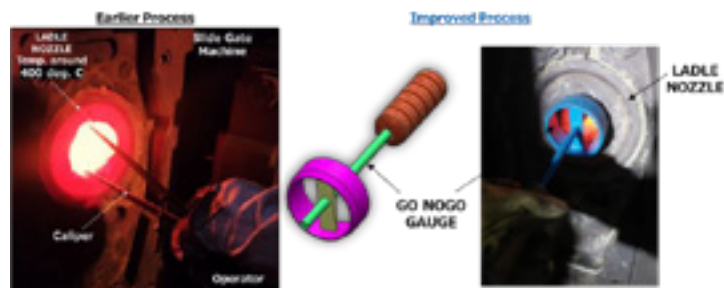
Fig. 7: Checking of Ladle Nozzle bore previous (with caliper and tape) VS now (with GO NOGO Gauge).
