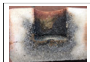
Fig. 13+14: Corundum stone with 99% Al_2O_3 , completely infiltrated and broken through
