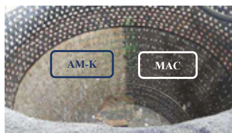
Fig. 5: Ladle barrel assembling for customer trial with MAC and AM-K lining with the zero carbon technology concept.
