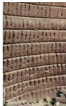
Fig. 2: Surface appearance of wear bricks at 2060 heats of service life.
