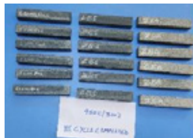
Fig. 3 : Samples after three cycles of Alkali Test
