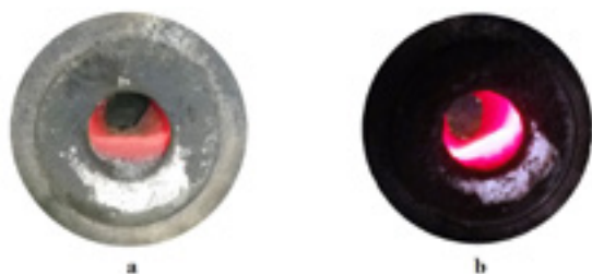
Fig. 9: a) - uniform filling of the worn area, b) - patching after reheating and erosion-corrosive wear.
