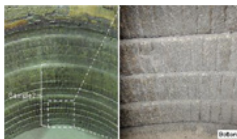
Fig. 10: Surface appearance of new ASC wear bricks at 1978 heats of service life.
