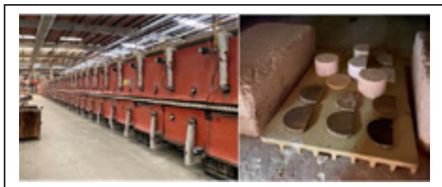
Fig. 10: Industrial roller kiln and coated samples that were introduced into the kiln.
