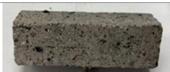
Sample of chamotte fireclay brick after test (95% CO and 5% H 2 )
