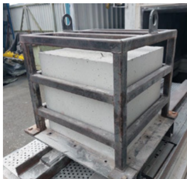
Fig. 5: Element after 30-hour drying time with 0.5 wt-% CAC content.
