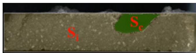
Fig. 2. Cross section of MgO-C refractory shape after a corrosion test in an induction furnace.
