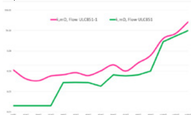
Figure 2 The permeability of Flow ULC 851 with/without special plant fiber after treated at different temperatures
