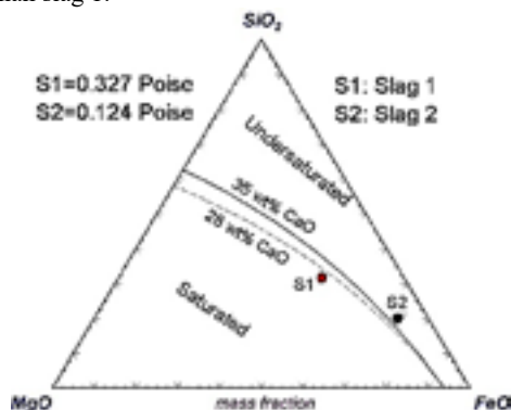
Fig. 3: MgO saturation lines of slags at 28% CaO and 35% CaO in the system \text{CaO-SiO}_2\text{-FeO-MgO-5\%Al}_2\text{O}_3 and slag viscosities calculated by Factsage at 1600 °C 1 atm.
