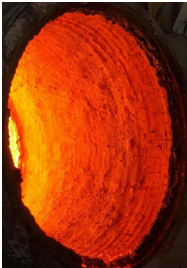
Fig. 6: Steel ladle repaired with ShotGun during operation
