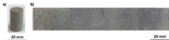
Fig 1. Single-sintered castable refractory composite specimens used for the compression tests (a) and bending tests (b).
