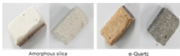
Fig.8 Specimen before and after hydrogen heat treatment
